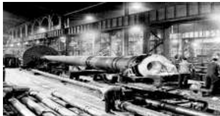
Final Bore alignment check after cutting 16" gun 1943 (2)
