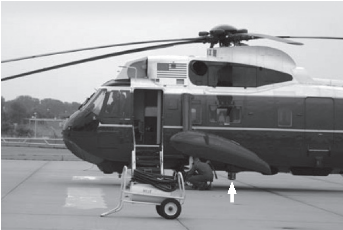
Marine One with AN/ALQ-144 IR CM System as indicated by the arrow. (Photo courtesy of William Kerr – National Geographic Channel)
