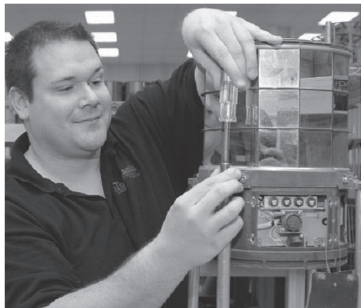
Disassembling the AN/ALQ-144 IR Jammer (Photo courtesy of Tobyhanna Army Depot)
