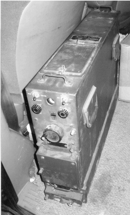
The BC-1073-A IFF Control Unit, as found
