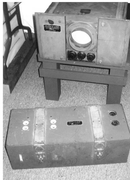
Top is the BC-941 Range Indicator to the SCR-547 Radar (Mickey Mouse)
